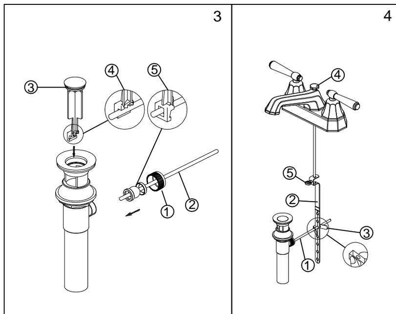
3. Remove pivot nut (1). Install horizontal rod (2) and stopper (3) as removable (4) or non-removable (5). Hand tighten pivot nut (1).
