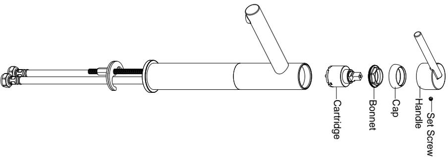
Many of these parts come preassembled. This exploded diagram is to assist in trouble shooting.
